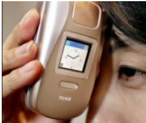
Figure 3. The TS41 Bone-Phone, which can transmit sound via the bone of the skull.
