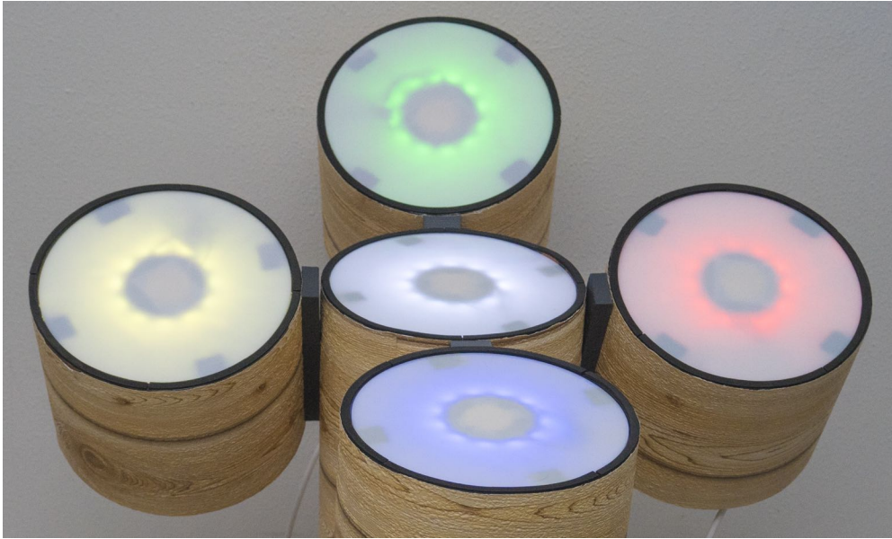
Figure 24. The circular shape seen in the middle of the drumheads, meant as a hint of where to hit the drums.
