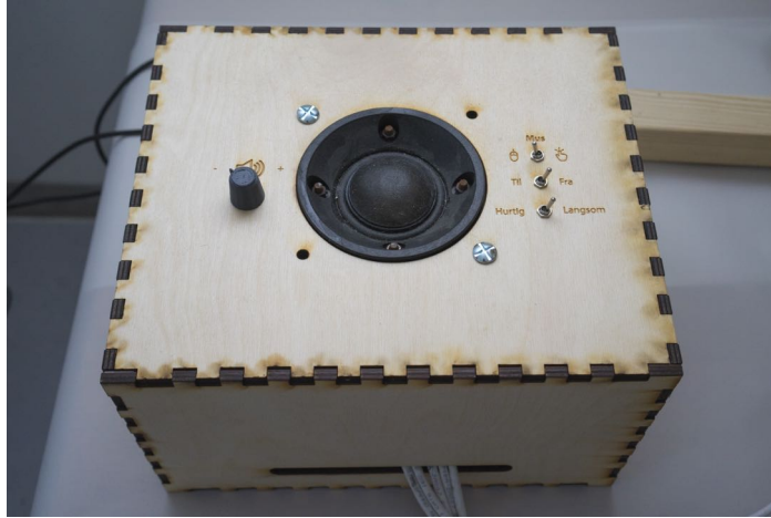
Figure 26. The control panel which is used to adjust the settings, while also containing the electronics.
