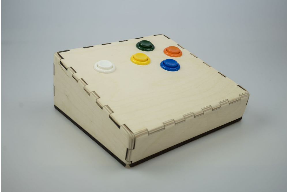
Figure 16. Second iteration of the developed traditional AT Prototype. As can be seen the edges are now softer, and the buttons are colored.
