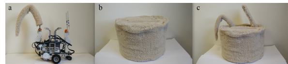
Figure 1. Then final prototype. a) Inner workings, b) Closed prototype and c) Protruded ears and tail.
